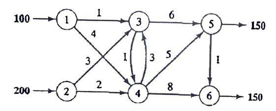
(v) Midwest TV Cable Company is in the process of providing cable services to five new housing development areas. The adjoining figure depicts possible TV linkages among the five areas. The cable miles are shown on each arc. Determine the most economical cable network starting at node 5.
